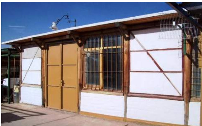
Fig. 9. Workshop with finished wattle and daub walls.
