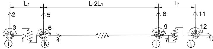
**Figure 6.** Column macro-element with nonlinear springs and degrees of freedom.
