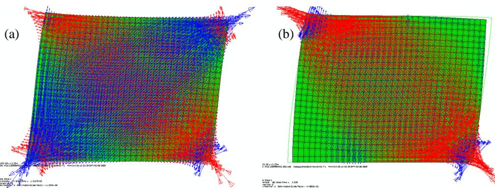
**Figure 1.** Principal stresses in the masonry wall, (a) before structural separation and (b) after separation (blue arrows indicate maximum principal stresses and red arrows minimum principal stresses).
