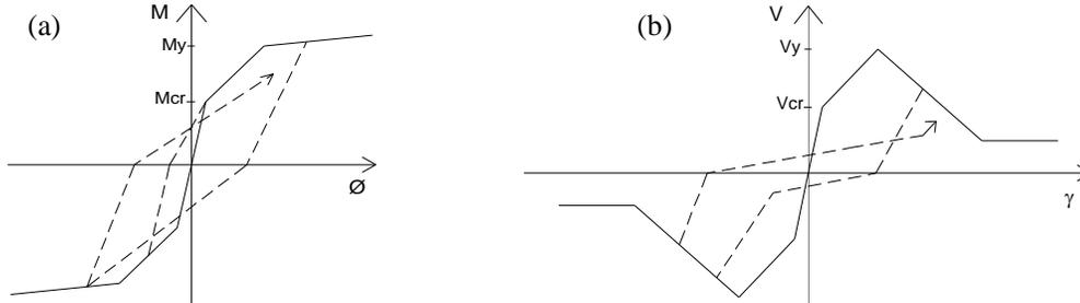
**Figure 7.** Hysteretic rules for (a) flexure and (b) shear.
