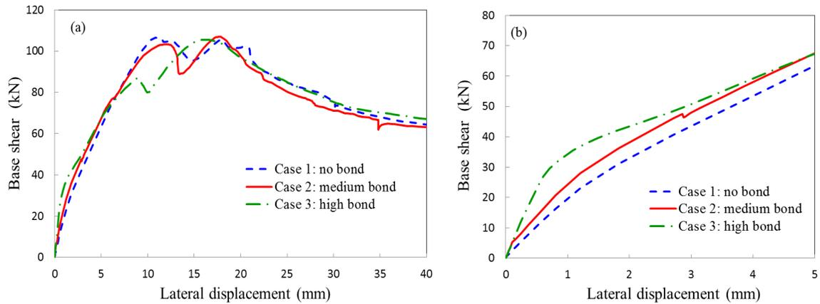
**Figure 4.** Force-displacement response for the three models, (a) complete response and (b) detail of the response in the range of small displacements.
