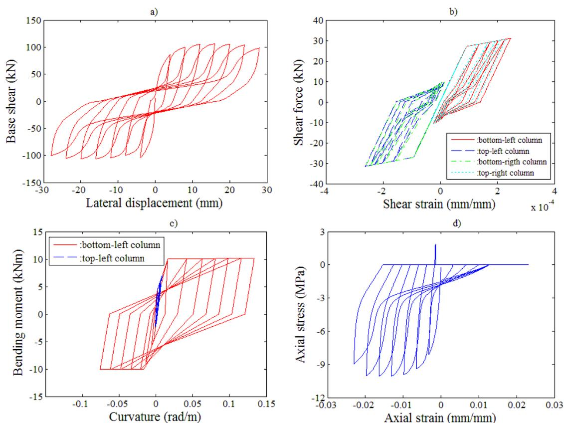
**Figure 9.** Computed response of a confined masonry wall, (a) global response, (b) shear response at the end of the columns, (c) flexural response of the left column and (d) response of the principal strut.
