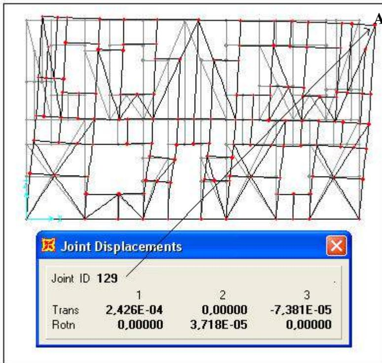
Figure 3.8. Displacements in 'himis' structure with brick infill under lateral loads
