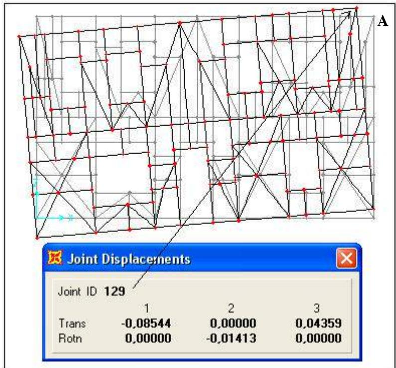
Figure 3.12. Displacements in 'himis' structure with brick infill in support settlement analysis
