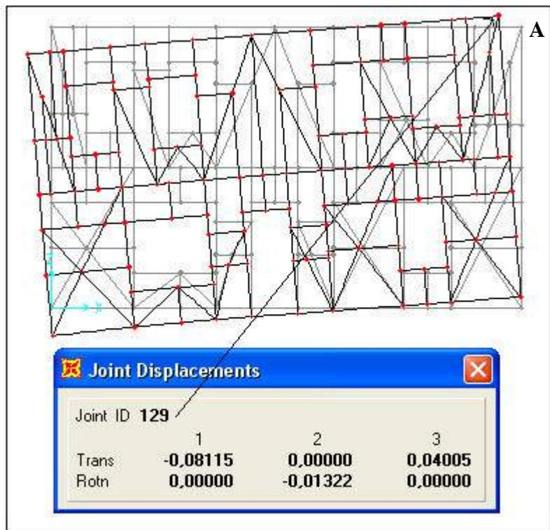
Figure 3.13. Displacements in 'himis' structure with adobe infill in support settlement analysis
