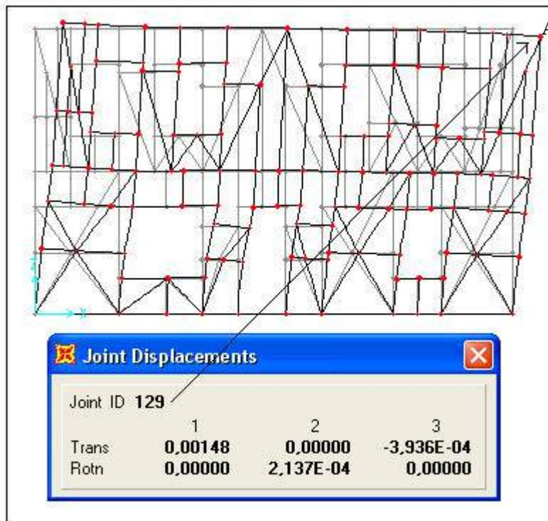
Figure 3.9. Displacements in 'himis' structure with adobe infill under lateral loads
