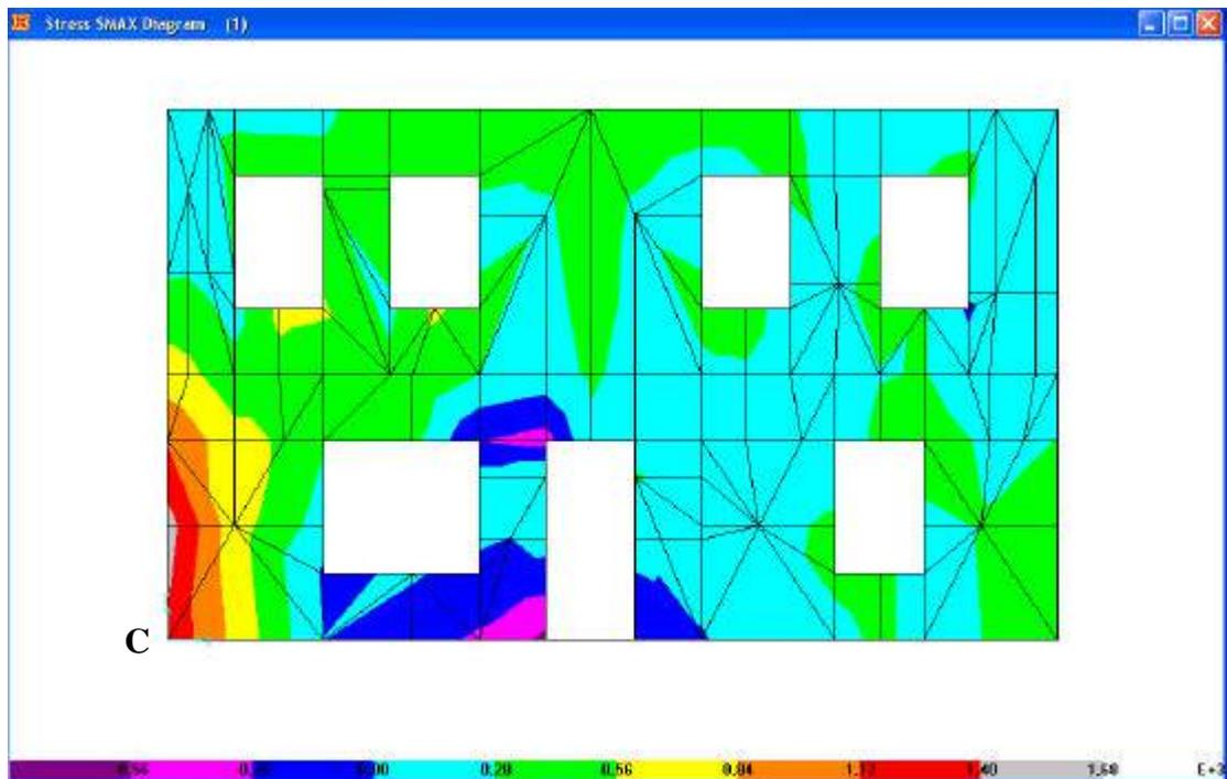
Figure 3.15. Stress distributions in 'himis' structure with adobe infill in support settlement analysis
