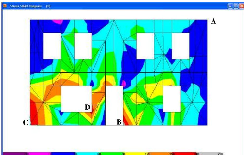
Figure 3.11. Stress distributions in 'himis' structure with adobe infill under lateral loads
