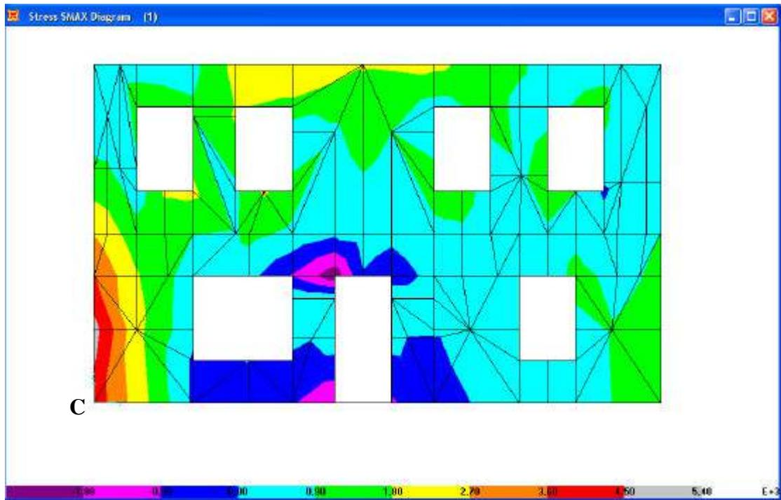
Figure 3.14. Stress distributions in 'himis' structure with brick infill in support settlement analysis
