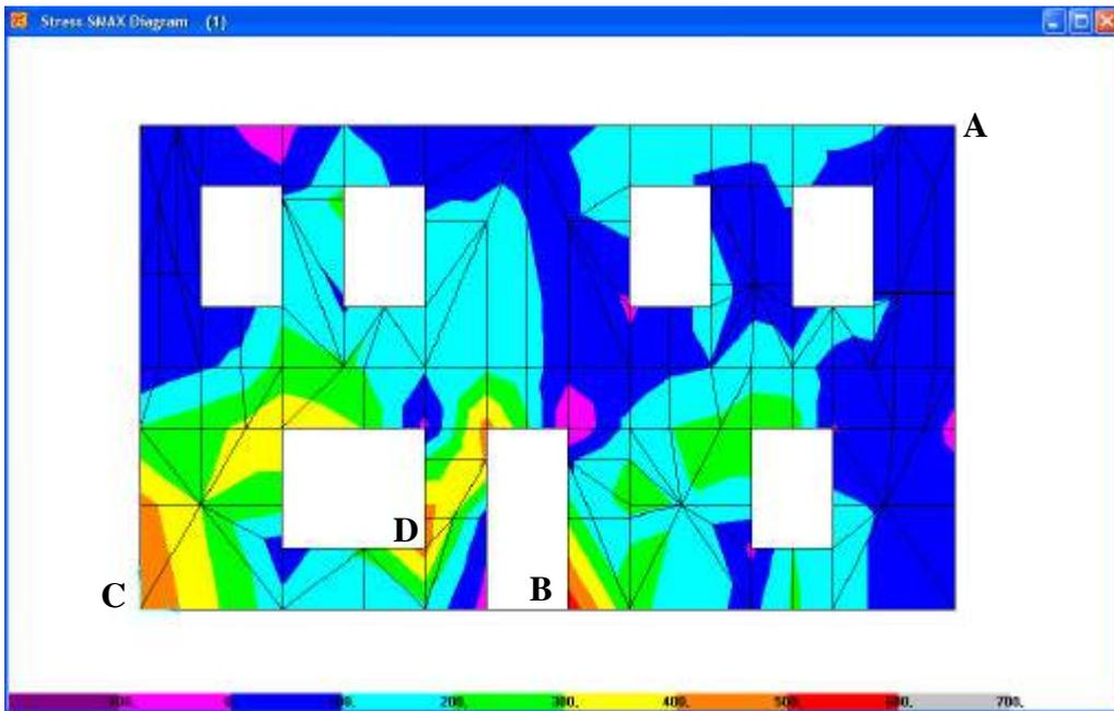
Figure 3.10. Stress distributions in 'himis' structure with brick infill under lateral loads
