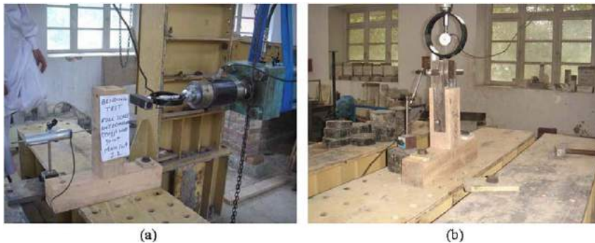
Figure 6. Set up for bending and tension tests on connection specimens: (a) Bending test and (b) tension test.
