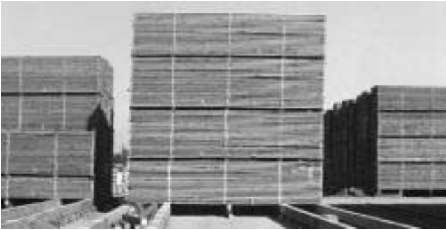
Figure 13–8. A sanitary, well-drained air-drying yard.
