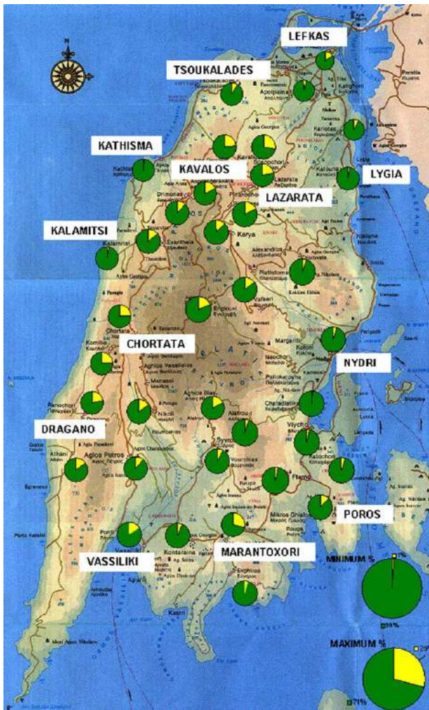
Fig. 8. Damage distribution of buildings in Lefkada island. The dark green portion of damage pies corresponds to unharmed, light yellow to buildings presenting some form of damage.
