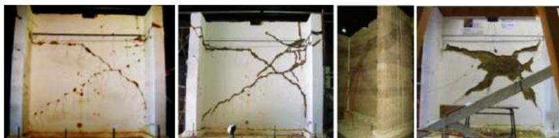
**Figure 10- Respectively from right to left U-shape model after first simulated cracking, after grouting, after reinforcing with mesh-band and final damage state [16].**
