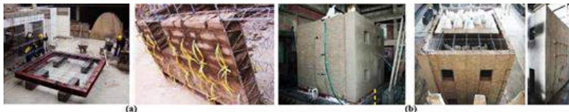
**Figure 5: (a) The process of adobe model's construction by ISM system; and (b) damages on adobe model reinforced with IM system after shake table test [11].**
