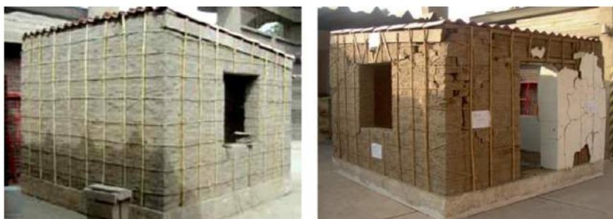
**Figure 2: An adobe-building model with external vertical cane and horizontal rope reinforcement (Source: (Left) [3]; and (Right) [5]).**
