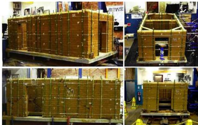
Figure 11: Specimen 4A after simulation of S8 [7].
