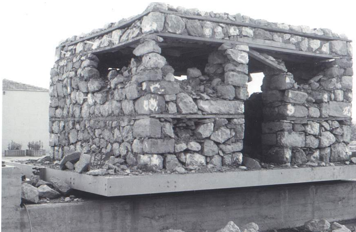
Photograph 2: The Cambridge-Ankara Shaking Table with Test House Model
