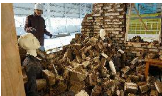
Model A: West and East walls collapsed due to out-of-plane loading; large cracks from window openings in North and South walls
