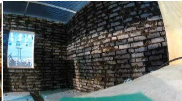
Model A: West and East walls collapsed due to out-of-plane loading; large cracks from window openings in North and South walls
