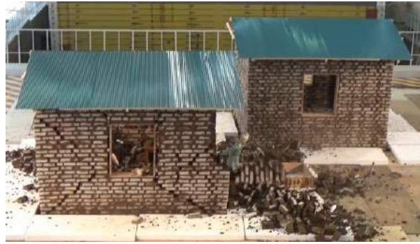
Figure 18: February 26, 2019 shaking table test: Model A collapsed & Model B still standing due to 70% JMA Kobe
