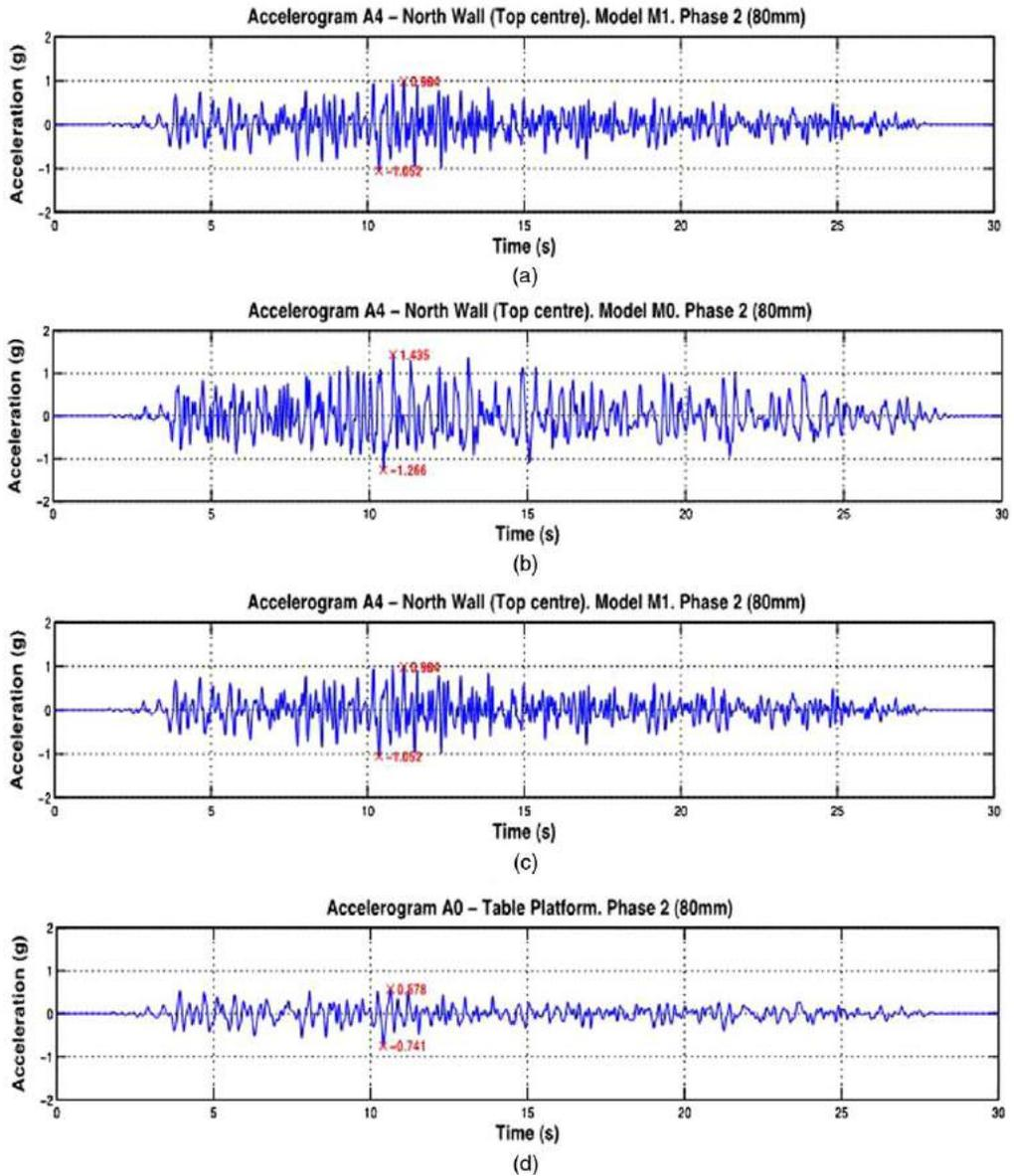
**Figure 27.** Recorded accelerations for phase 2—top north wall.
