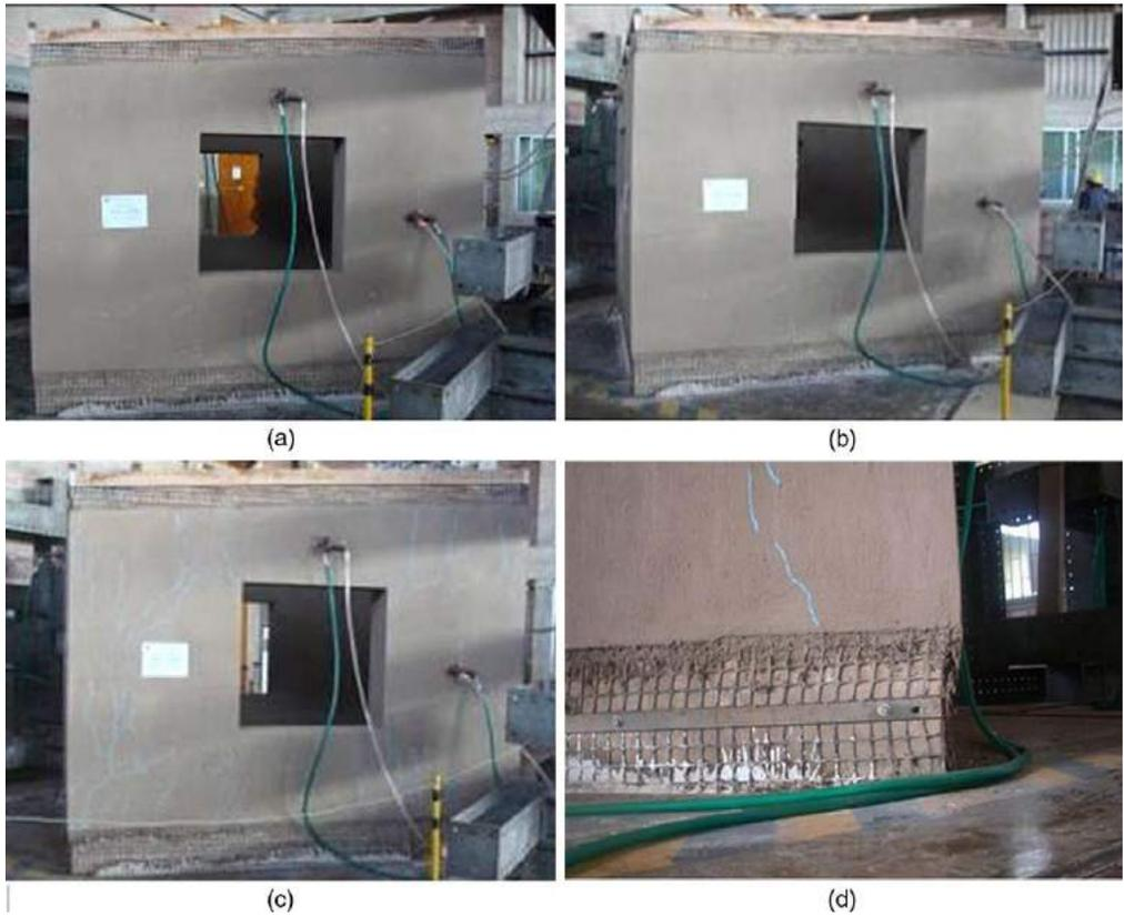
**Figure 25.** Damage in model M2: (a) Post-phase 1; (b) post-phase 2; (c) post-phase 3; (d) post-phase 3.
