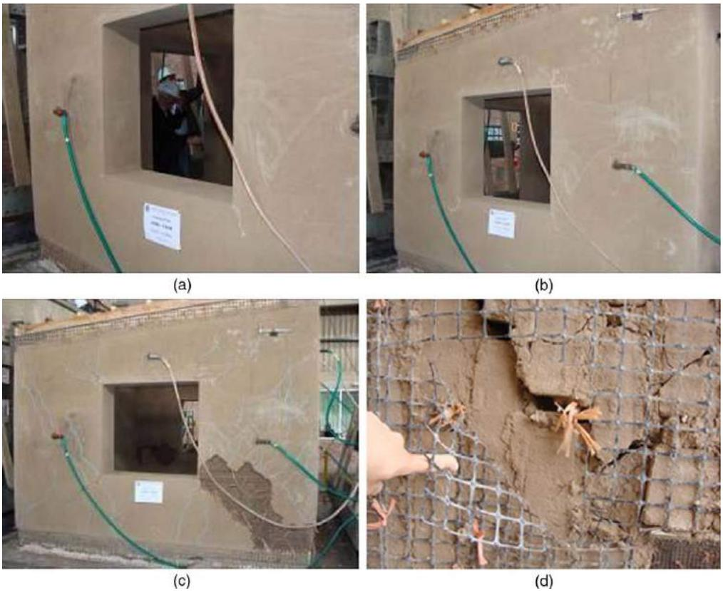
Figure 23. Damage in M1 model: (a) post-phase 1; (b) post-phase 2; (c) post-phase 3; (d) geogrid failure.
