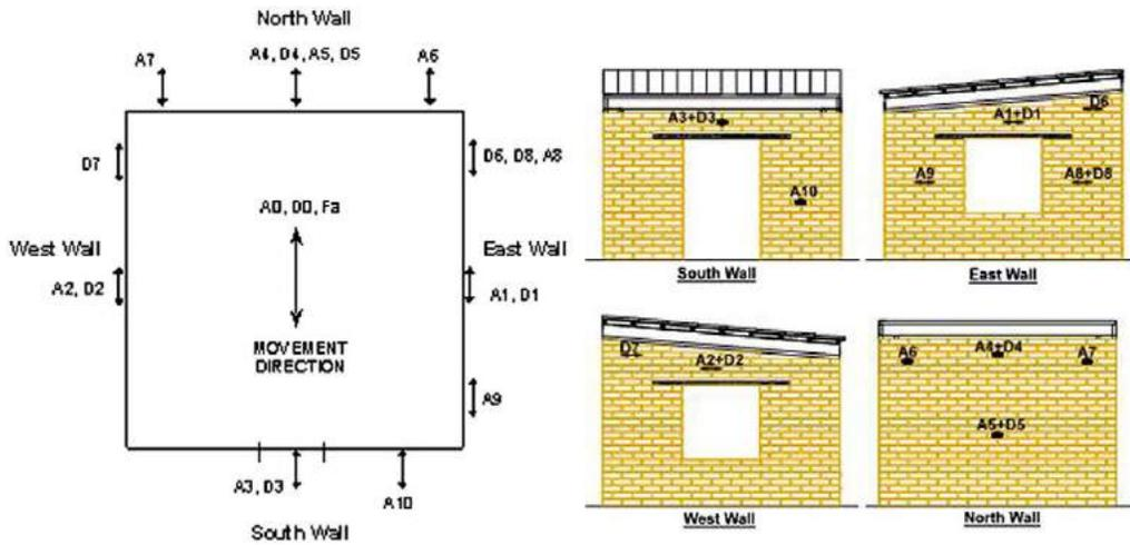
**Figure 18.** Ground plan and elevation distribution of instruments in models M0 and M1.
