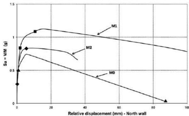
**Figure 29.** Lateral force vs. relative displacement envelope—north wall.
