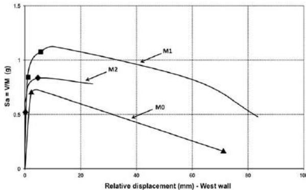
**Figure 28.** Lateral force vs. relative displacement envelope—west wall.
