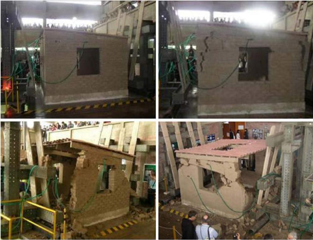
**Figure 21.** Damage in model M0.
