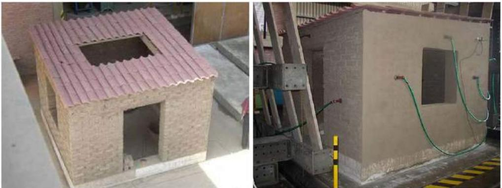
**Figure 20.** Unreinforced model—M0.
