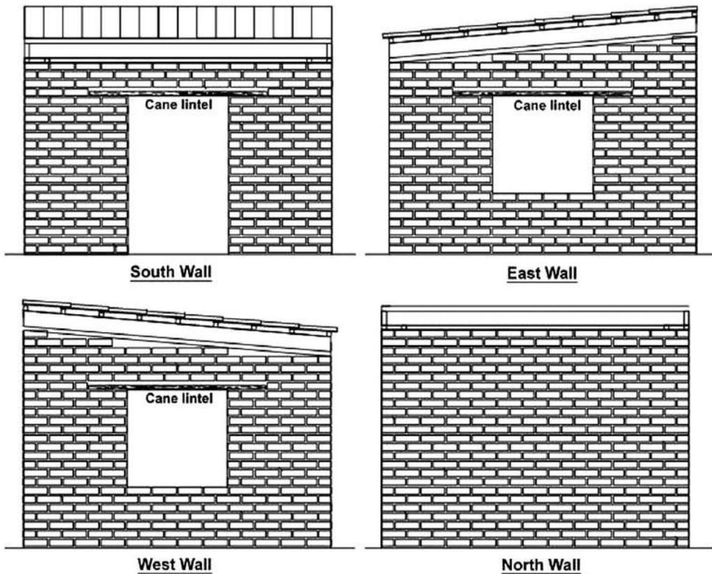
**Figure 3.** Elevation of walls: (a) south wall; (b) east wall; (c) west wall; (d) north wall.
