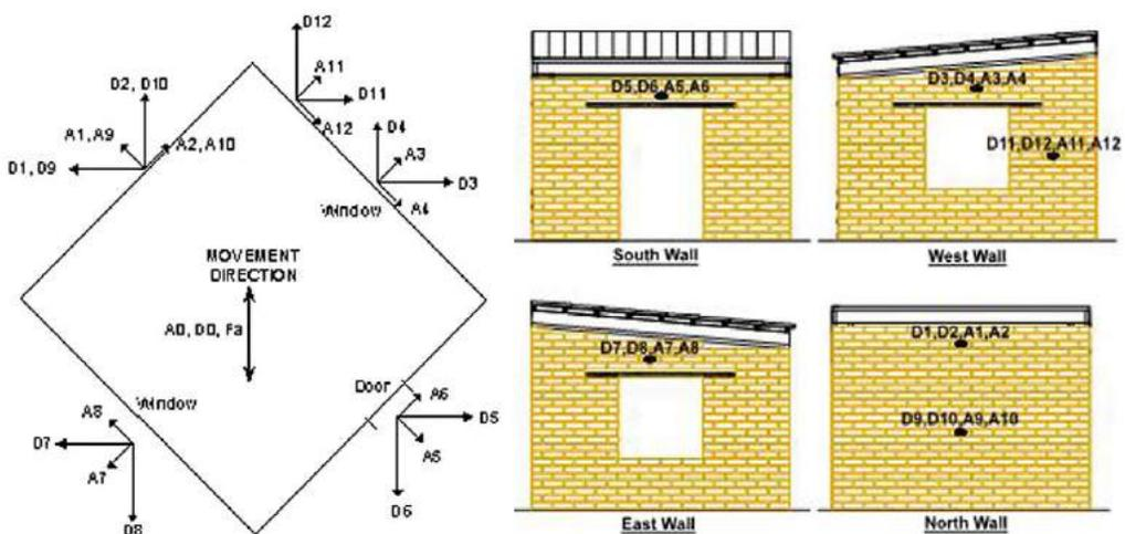
**Figure 19.** Ground plan and elevation distribution of instruments in model M2.
