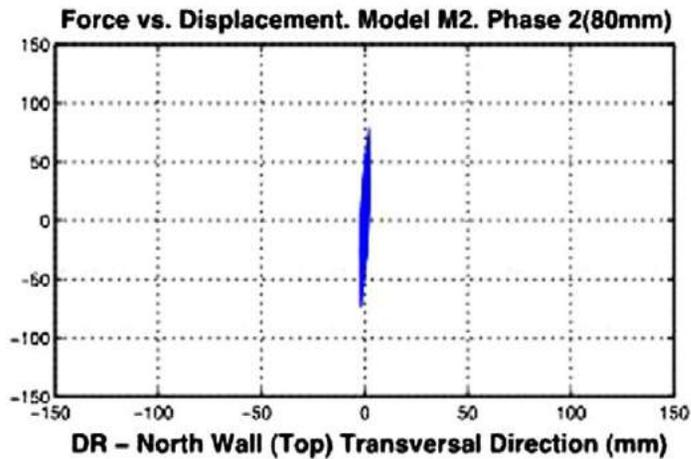
**Figure 26.** Lateral force vs. north wall top displacement, phase 2 (80 mm peak table displacement): (a) unreinforced model (M0); (b) Reinforced model (M1); (c) reinforced model (M2).
