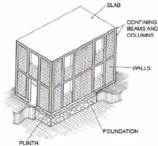
Figure 1: A typical confined masonry building [3].
